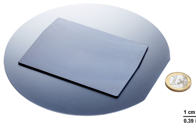
Fig. 1. CdZnTe substrate on a 6'' (c.15-cm) Si wafer before polishing and a one Euro coin for size comparison. The wafer's dimension is 65\text{ cm}^2 .
