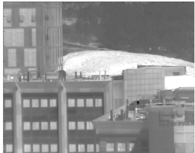
Fig. 13. Image registered with a demonstration camera containing the 15- \mu\text{m} pitch, 640 \times 512 Pelican-D LW FPA, operating with improvised (non-optimum) F/2.7 optics at 77 K.
