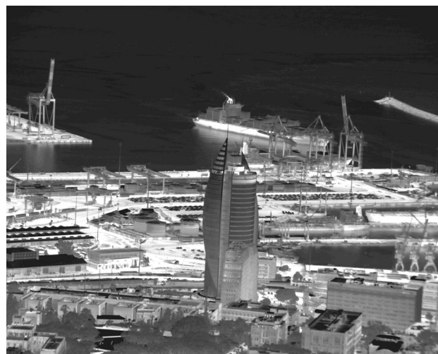
Fig. 5. Image registered with a 1280 \times 1024 HOT Hercules XBn FPA at F/3 and 150 K.
