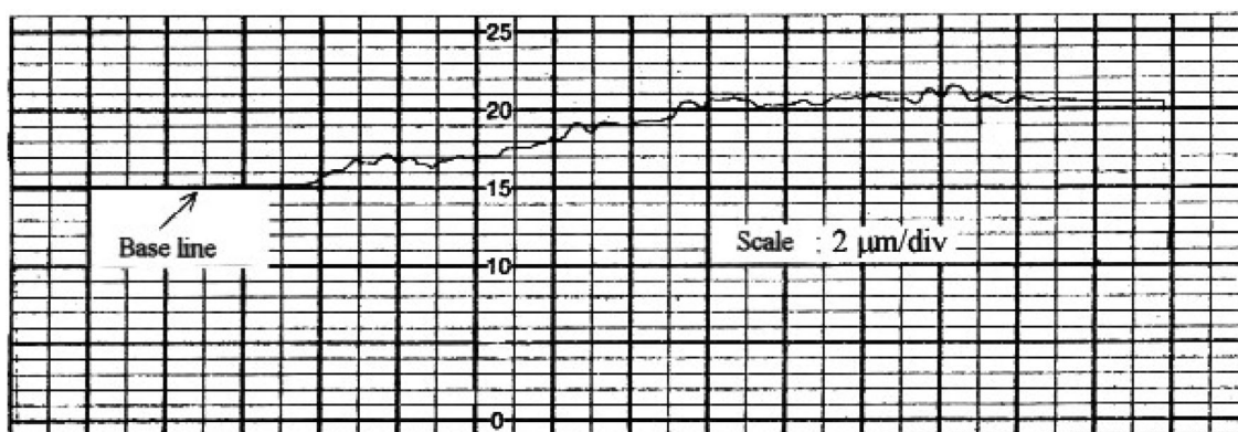
Fig. 1. Talystep profile of \text{In}_2\text{S}_3 film.
