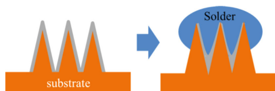
Fig. 12. Schematic diagram of interfacial void disappearance.
