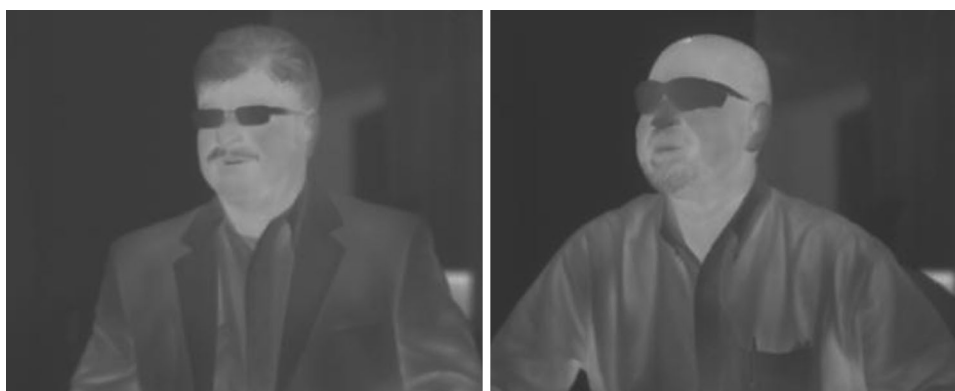
Fig. 5. Thermal images taken by use of a 320 × 256, 30 μm pitch MWIR HgCdTe/CdTe/Si FPA operating at 85 K (frame rate 60 Hz, integration time 1 ms).
