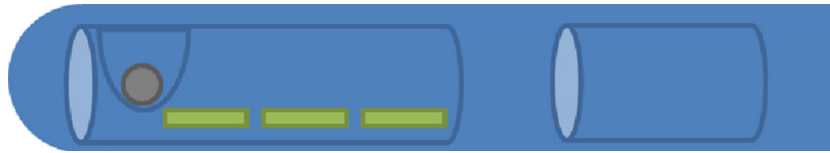
Fig. 1. Ampoule schematic showing samples, plug and mercury placement. Gray circle represents Hg. Green bars represent MCT samples. Design is not drawn to scale.
