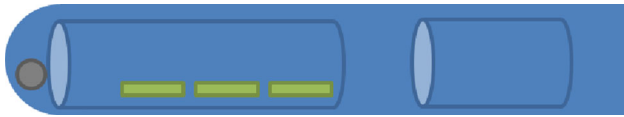
Fig. 10. Original ampoule design with mercury placed at the end of the ampoule and samples placed on a carrier.
