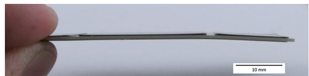
Fig. 5. Photograph of 8/25/8 mil AlN DBC sample after 100 cycles showing cracking and bowing of substrate.
