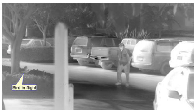
Fig. 10. Video screenshot obtained from band 2 (LWIR) using a camera built with a wafer produced in this work.
