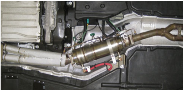
Fig. 5. TEG integration into the exhaust line of the BMW X6 prototype vehicle.
