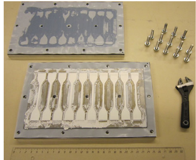
Fig. 2. The opened mold with ten cured samples in the slots. It consists of two 9.5-mm-thick aluminum plates, two 2-mm-thick rubber sheets, two 0.25-mm-thick PTFE sheets, and a 2-mm-thick steel plate.
