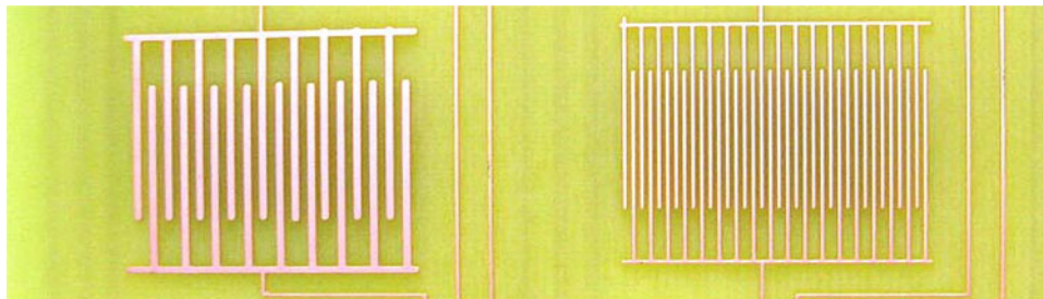
Fig. 1. Image of a test board prior to soldering, containing comb structures based on an IPC B-24 pattern, with 0.64 mm (25 mil, left) and 0.32 mm (12.5 mil, right) conductor spacings.
