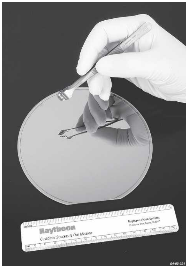
Fig. 1. Photograph of a 6-in diameter HgCdTe/Si wafer.
