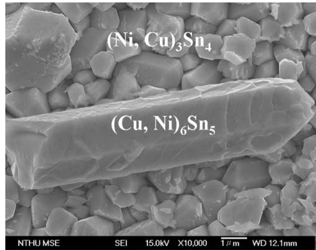
Fig. 8. Top-view morphology of IMCs in the Sn-37Pb solder/Ni/Cu joints reflowed at 245°C for (a) three and (b) ten cycles.
