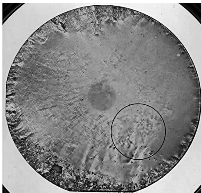
Fig. 2. The circular-linear polarized image of the same 2-in.-diameter, 4H-SiC PIN diode wafer shown in Fig. 1. The top polarizer (at the light source) is circular, while the analyzing polarizer (at the CCD detectors) is linear. Note that the area outside of the wafer is bright because this configuration does not extinguish all of the light. The circle indicates the region in which Raman analysis was performed.
