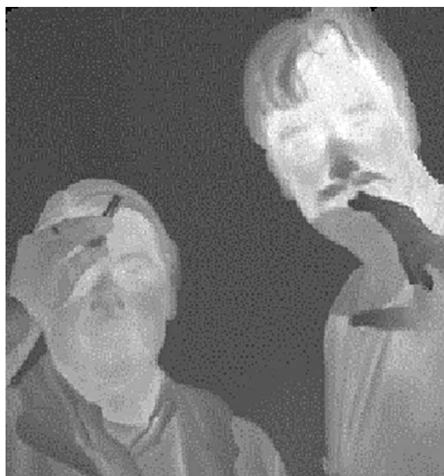
Fig. 8. Image produced by FPA from layer 3-1085 operated in an IR camera with f/2 optics and 52 Hz frame rate.
