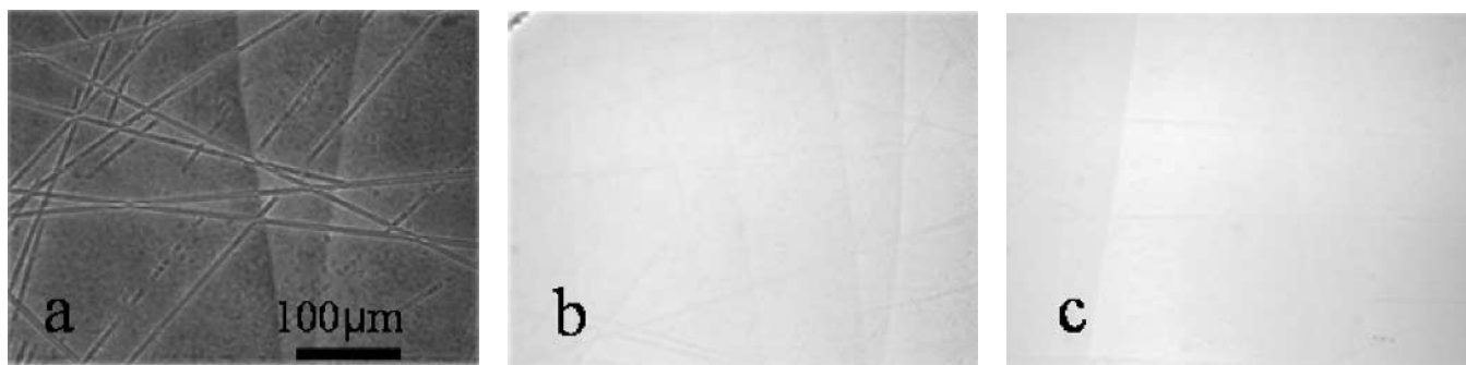
Fig. 3. Optical microscope images of an oxidized surface under 5\text{ mA/cm}^2 for 30 sec after (a) 1 cycle, (b) 6 cycles, and (c) 12 cycles of polishing using the two-step ECMP process.
