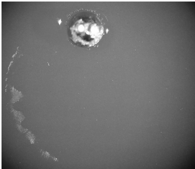
Fig. 6. An example of solder-paste B after reflow in (a) air and (b) nitrogen atmosphere.
