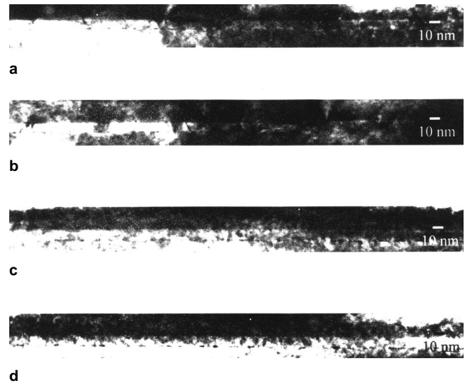
Fig. 3. Bright field [110] XTEM image of (a) the as-grown 5% BSG sample, (b) the 5% BSG sample annealed at 850°C for 30 min in nitrogen ambient, (c) the as-grown 20% BSG sample, (d) the 20% BSG sample annealed at 850°C for 30 min in nitrogen ambient.
