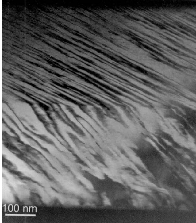
Fig. 2. [110] transmission electron microscopy cross section of a sample where the lower layer was undoped and the upper layer was grown having a DETe flow rate consistent with a Te doping level of 4 \times 10^{17} \text{ cm}^{-3} . A clear change in the APB spacing and angle is seen at the interface, where growth was interrupted for 10 sec while Te was added to the system.
