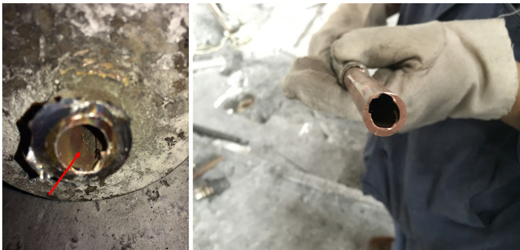
Fig. 12—Lance worn out in the industrial experiment.
