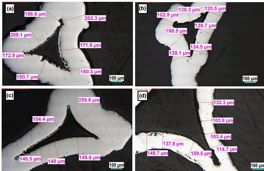
Fig. 1—Cross-sectional optical images of (a) foam surface and (b) core by DC condition and (c) foam surface and (d) core by PCcondition.
