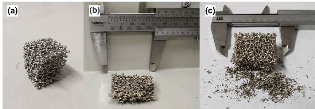
Fig. 7—(a) Ni/SiC foam sample before compressive test, (b) non-composite nickel foam after compressive test, (c) composite foam after compressive test.
