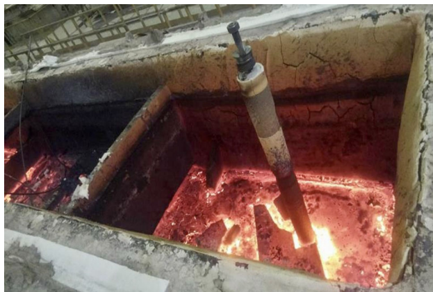
Fig. 2—Photo of the tundish refractory lining after one casting period.
