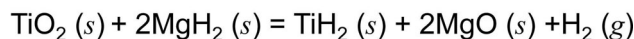
Fig. 8—Schematic illustration of the reaction system in the hydrogen-assisted magnesiothermic reduction (HAMR) process. [62]
