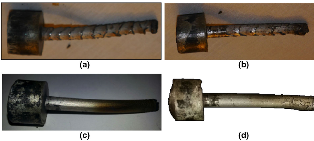
Fig. 5—Extrudates extruded at temperatures in the \alpha -Ti phase field (806 °C) (a) CP-Ti, (b) UAT-Ti, and in the \beta -Ti phase field (1234 °C) (c) CP-Ti and (d) UAT-Ti.
