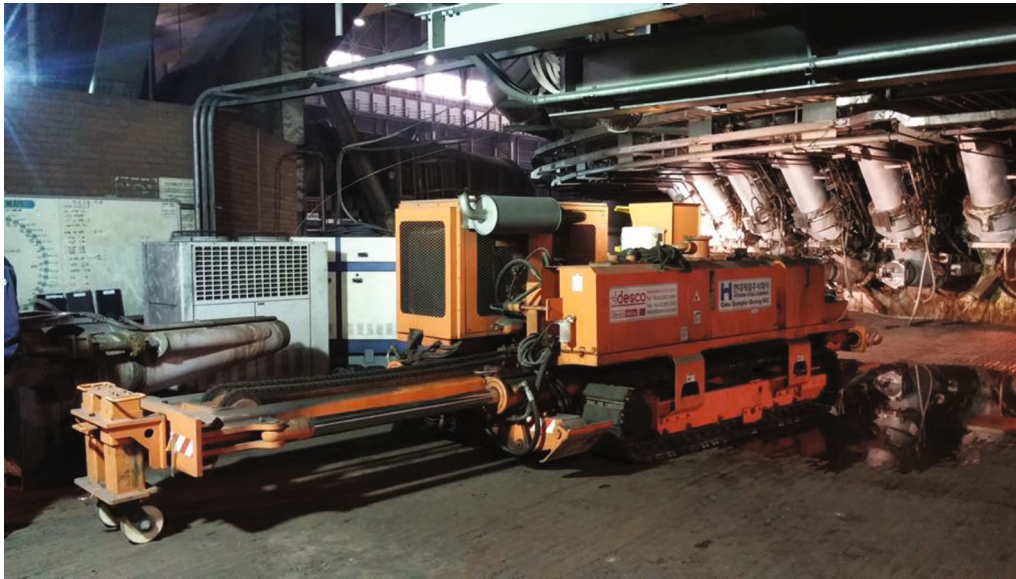
Fig. 1—Schematic diagram of the drilling equipment used to extract the coke samples at the tuyere.
