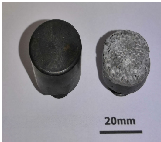
Fig. 8—Image of the AISI 4340 sonotrode before and after it was used for UST (Color figure online).
