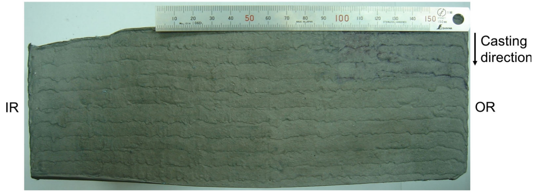
Fig. 4—Oscillation mark profiles on the steel slab: narrow face view.
