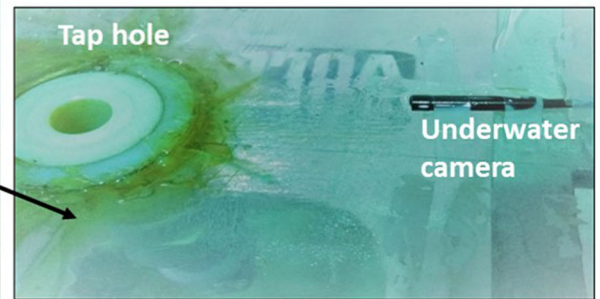
Fig. 2—(a) Schematic and (b) pictorial representation of the fabricated Perspex BOF model for tapping study, (c) side view of the fabricated BOF model, and (d) arrangement of an underwater camera to monitor the vortex and drain sink events.
