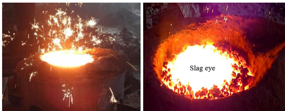
Fig. 6—Experimental photos of the bottom powder injection process in the 2-t medium frequency induction furnace.
