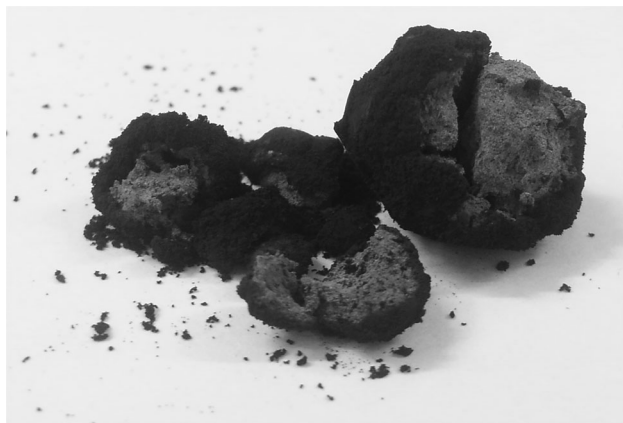
Fig. 5—Carbon deposition in type B pellets reacted for 120 min at 1123 K (850 °C) in H 2 -CO.
