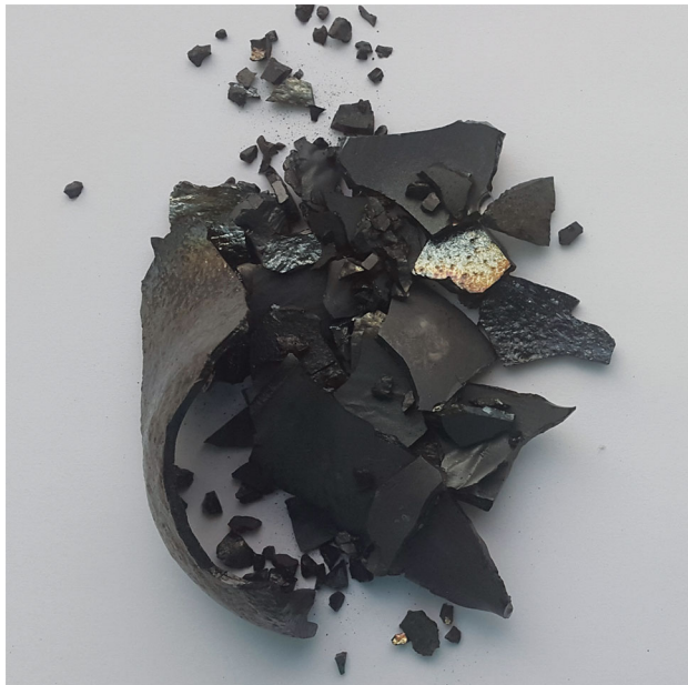
Fig. 3—The slag sample #10 taken during slag tapping.
