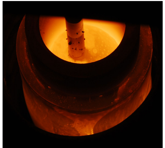
Fig. 2—Photo showing slag foaming.
