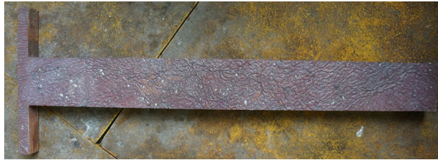
Fig. 2—The specially cut copper anode used in the copper electrorefining experiments.
