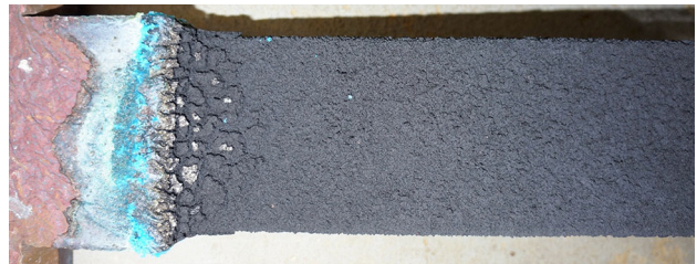
Fig. 4—The harvested anode with adhered anode slimes after the copper electrorefining experiment.
