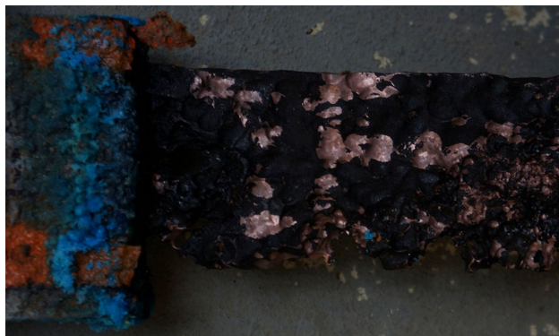
Fig. 5—The harvested anode with distinct surface morphologies after copper electrorefining Test-6.
