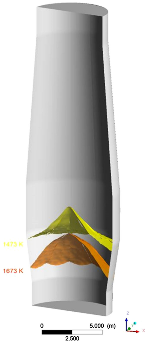
Fig. 5—Boundaries of cohesive zone determined by the simulation.
