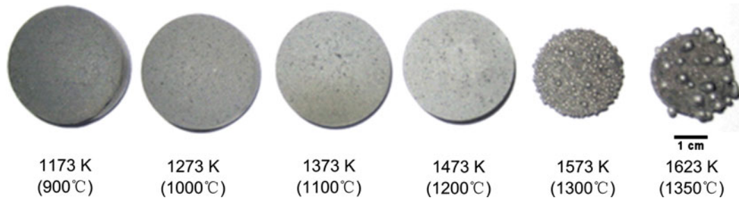
Fig. 11—Overall view of reduced coal-mixed PTC briquettes.
