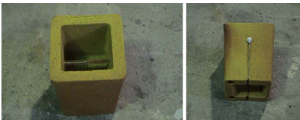
Fig. 6—QuickK-Cup sample containing K-type thermocouple. Cup dimensions are height = 58 mm, thickness = 7 mm for lateral and bottom walls.
