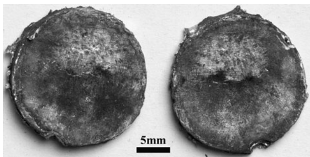
Fig. 13—Photograph of the oxide layers that were held in the liquid metal for 30 min. The dark area expanded over many parts of the oxide layer.
