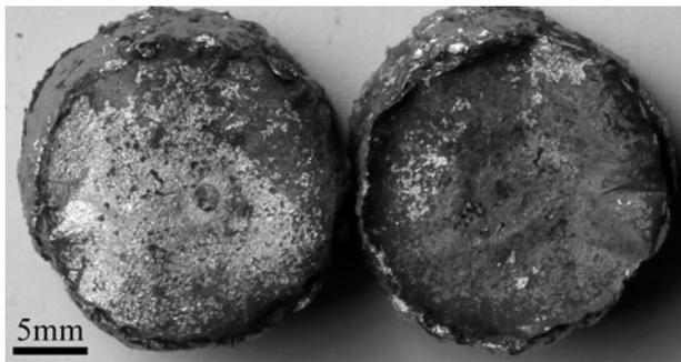
Fig. 14—Photograph of the oxide layers that were held in the liquid metal for 16 h, showing vast white areas on one side, which matched with vast darker areas on the other side.
