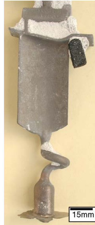
Fig. 9—Photograph of a blade with attached HC after shakeout from the mold.
