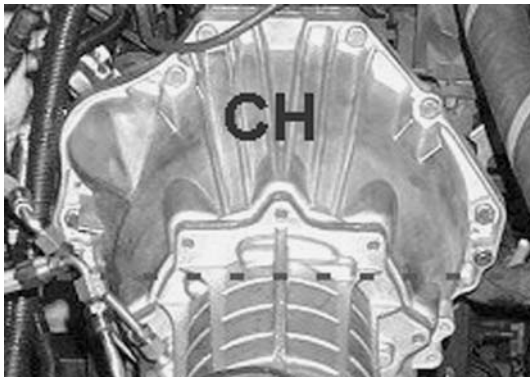
Fig. 2—Automotive converter housing part (marked CH) chosen for the LCA study.
