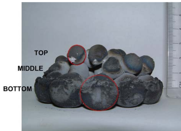
Fig. 11—Front view of reduced bed, involving reduction of a three-layer arrangement of the bed of PAH-wood-charcoal pellets, showing shrinkage and swelling of the different layers.
