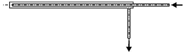
Fig. 3—Schematic drawing of the water-cooled probe. The arrows indicate the direction of the water flow.
