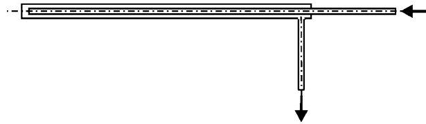
Fig. 3—Schematic drawing of the watercooled probe. The arrows indicate the water flow.
