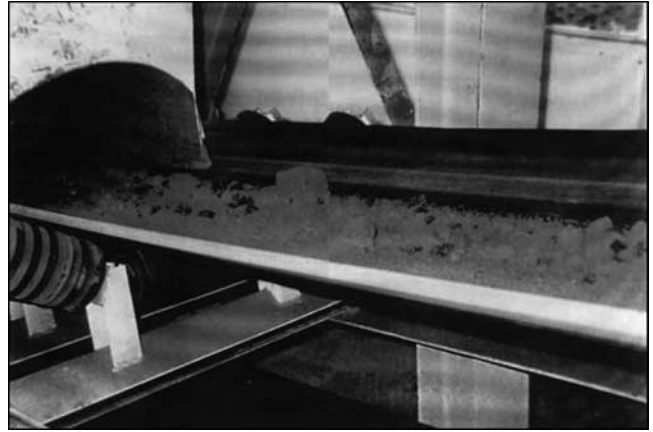
Fig. 15—Korea Zinc Co. Residue Fuming Plant feed. Little or no feed preparation is needed for Ausmelt furnaces.
