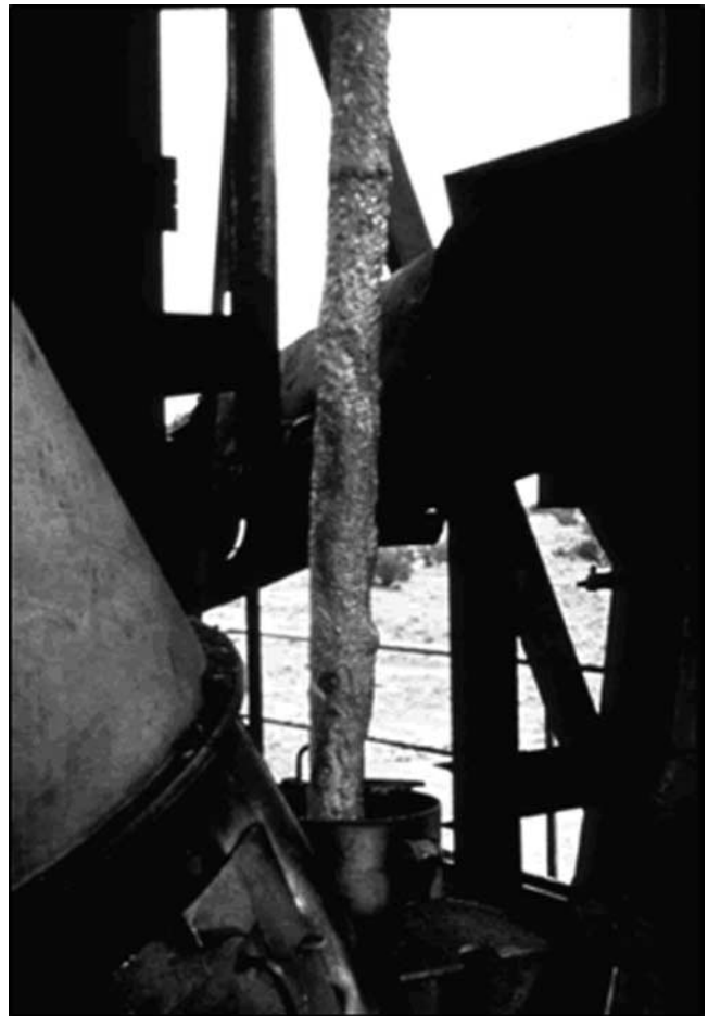
Fig. 11—Slag-coated lance being raised from the Olympic Dam reactor.
