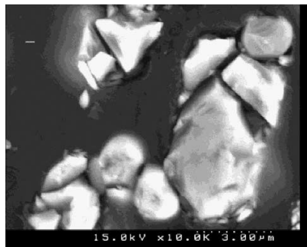
Fig. 8—SEM image of chromium oxide Cr 2 O 3 before reduction.
