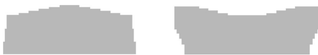
Fig. 1—Microscopic surface topography in the case of BCF-controlled growth (left) and VKS-controlled growth (right) (adapted from Ref. 17.)
