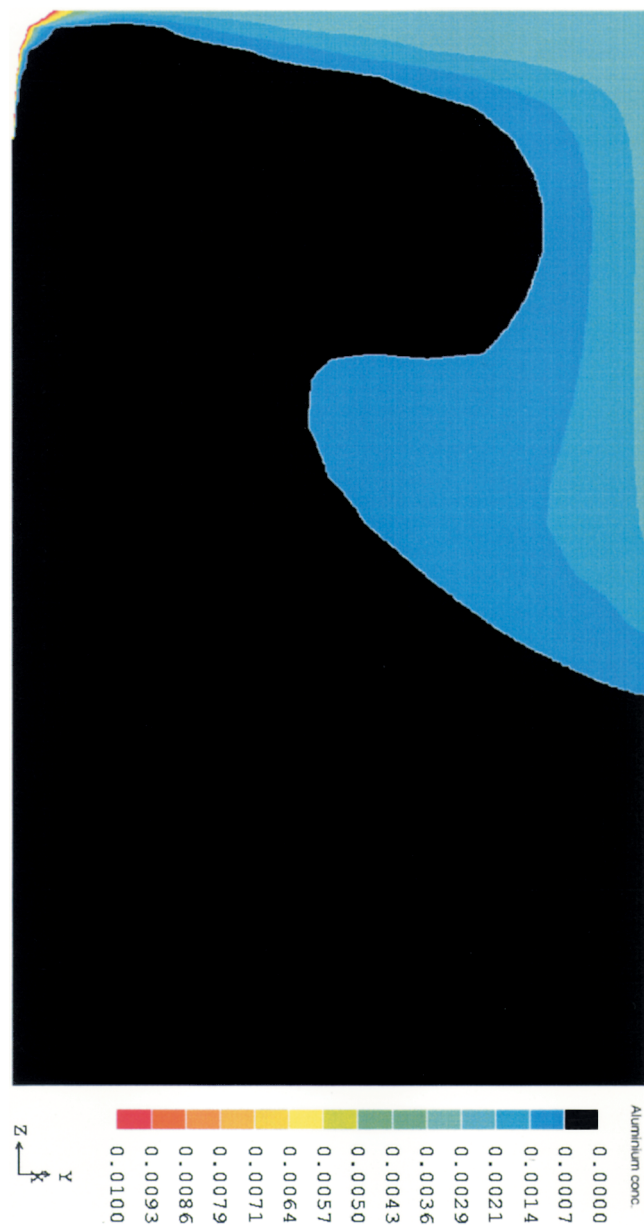
Fig. 5—Aluminum concentration at the end of wire injection, time = 30 s.
