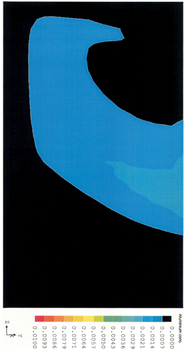
Fig. 8—Aluminum concentration after wire injection, time = 50 s.
