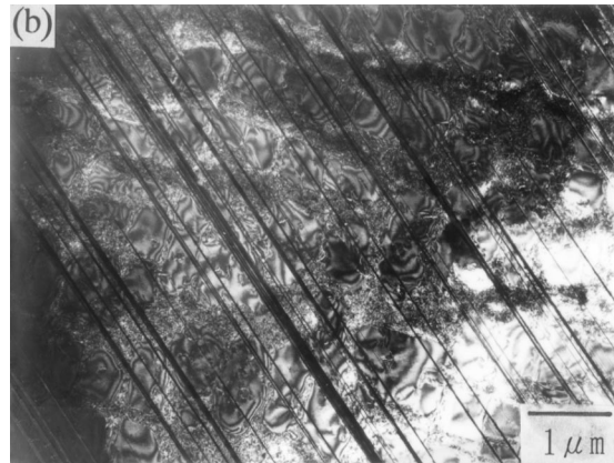
Fig. 13—TEM micrographs of the ruptured [011] specimen showing microtwin lamellae ( \epsilon = 9.6 pct). The foil normal is [0\bar{1}1] . (a) Bright-field micrograph. (b) Dark-field micrograph using spot 1. (c) Dark-field micrograph using spot 2. Shear strain for the (111)[\bar{2}11] slip system is 20.4 pct.
