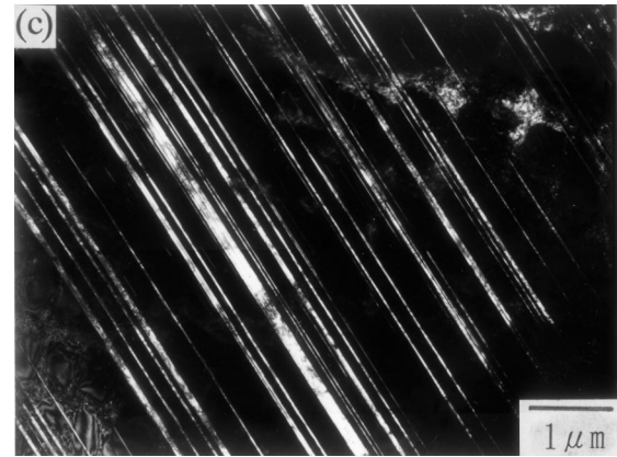
Fig. 13—TEM micrographs of the ruptured [011] specimen showing microtwin lamellae ( \epsilon = 9.6 pct). The foil normal is [0\bar{1}1] . (a) Bright-field micrograph. (b) Dark-field micrograph using spot 1. (c) Dark-field micrograph using spot 2. Shear strain for the (111)[\bar{2}11] slip system is 20.4 pct.
