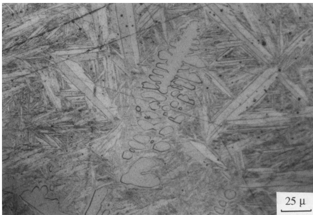
Fig. 5—The early stage of dendritic precipitation in a Cu-Al sample isothermally reacted at 750 °C for 5 min and then quenched in ice water.
