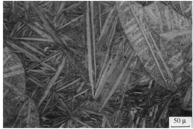
Fig. 2—Martensitic structure obtained in a Cu-Al sample quenched in ice water from 950 °C. The structure clearly shows the absence of original cast structure.
