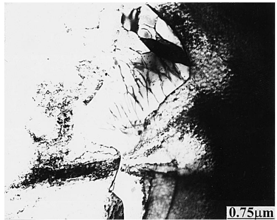
Fig. 3—MC carbide on the grain boundary of no. 1 alloy.
